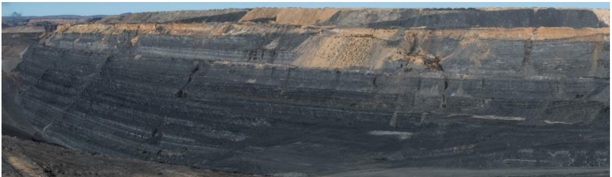
Plate 4-5: Main Series Pit high wall from the north west showing consistency of strata in the exposed Main Series Overburden.
