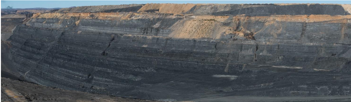
Figure 3. Main Series Pit highwall from the north west showing consistency of strata in the exposed Main Series Overburden. At its lowest point, the highwall is up to 180 m high.
