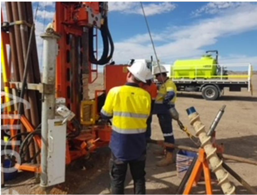
Drill rigs and teams geotechnical investigations associated with the construction of the NRUP) gasification wells and power generator areas.
